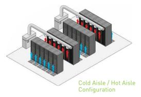
into a return air plenum. Hot aisle containment can provide 40% more savings than cold aisle/hot aisle configuration alone.
